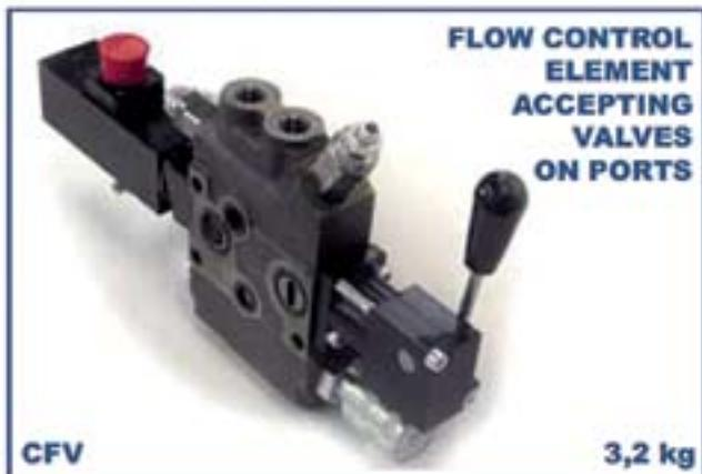
CF and CFV elements integrate a pressure compensated flow control that allows the external regulation of the flow inside the elements themselves and recuperates the exceeding flow (EF) for the following elements.
